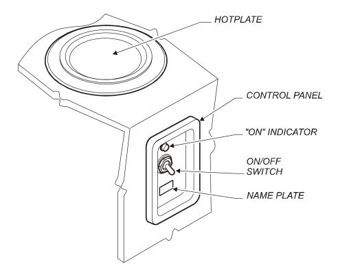
Fig 1. H-006UL Features and Operating Controls
